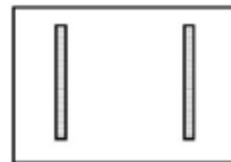
2. Because the black paper is conductive, potential difference between the electrodes sets up an electric field in the paper between them. You will be able to measure the potential rise/drop between any two points using two probes that are connected to a digital multimeter. You will use the multimeter as a voltmeter, which measures the potential rise/drop between its terminals. It is calibrated in volts with several scale settings.
