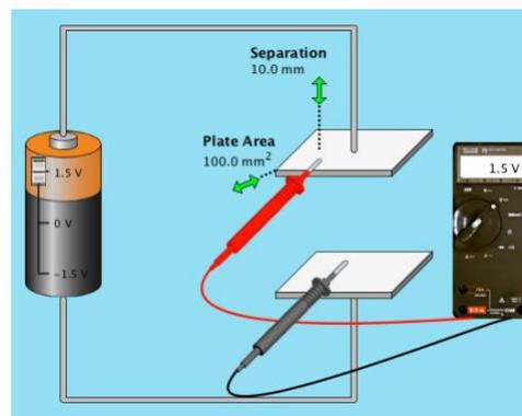
Draw below a capacitor (keep the plates horizontal as in the simulation) and draw (clearly indicate) the electric field lines in the region between the plates. Explain your reasoning. Use the data provided by the applet and calculate the strength (magnitude) of the electric field between the plates.
