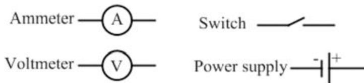
A current at any point in a circuit can be measured with an ammeter. Potential rise or drop in a circuit can be measured using a voltmeter.
