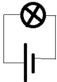
13. Connect another bulb (identical with the first one) in parallel with the first bulb, and check your prediction.
