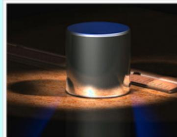
The **International Prototype Kilogram (IPK)** is an artifact standard or prototype that is defined to be exactly one kilogram mass.
